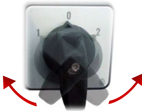
Figure 4. Main Control Switch
